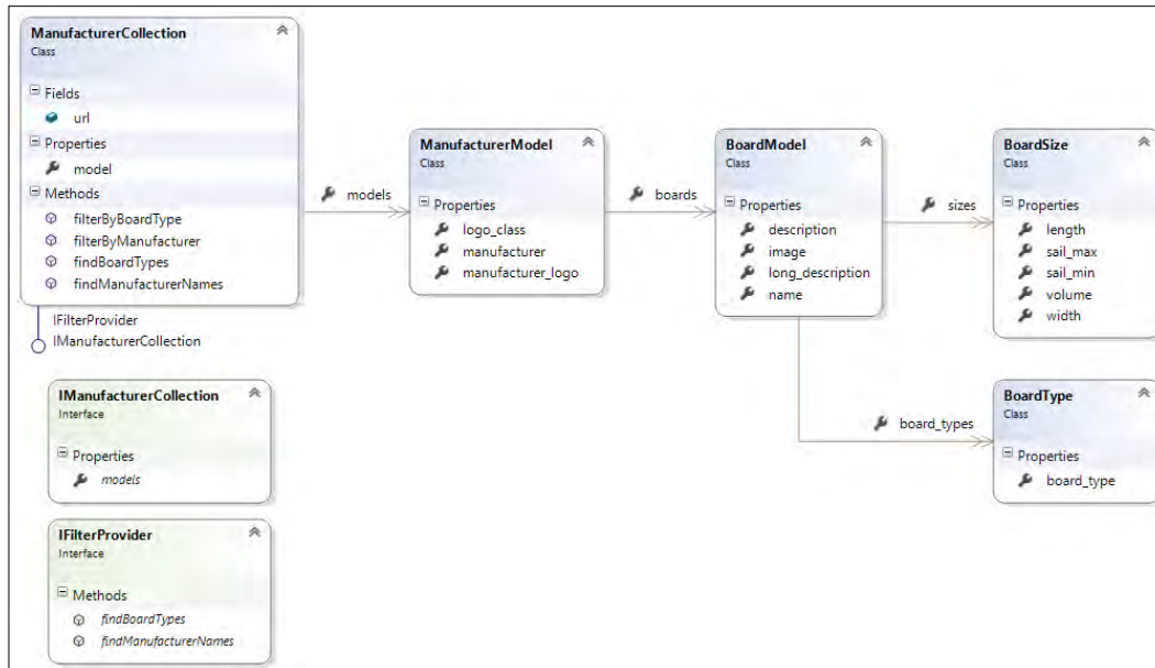
Class diagram of ManufacturerCollection and related Backbone models
